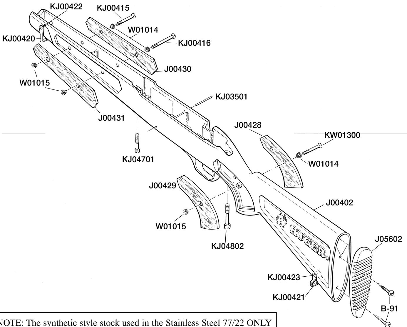
NOTE: The synthetic style stock used in the Stainless Steel 77/22 ONLY fits the stainless steel model. Neither the stock nor its fittings are interchangeable with corresponding parts of the blued 77/22 model.
